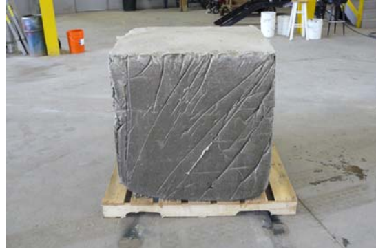
Above: A 3-ft by 3-ft by 3-ft (1 cubic yard) sample of the specified cement grout. As standard protocol, contractors are often asked to demonstrate calibrated settings. Note the completeness of the void fill and consistent nature of the grout produced by CRC's volumetric mixers.
